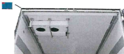
Second roof evaporator in the multi-temperature box.
