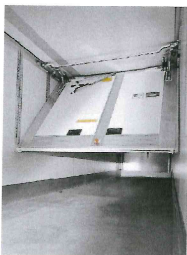
Two temperature zones: Adjustable, swivelling partition.
