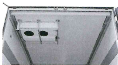
Second roof evaporator in the multi-temperature box.
