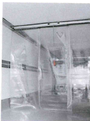
The adjustable strip curtain minimises cooling air loss.
